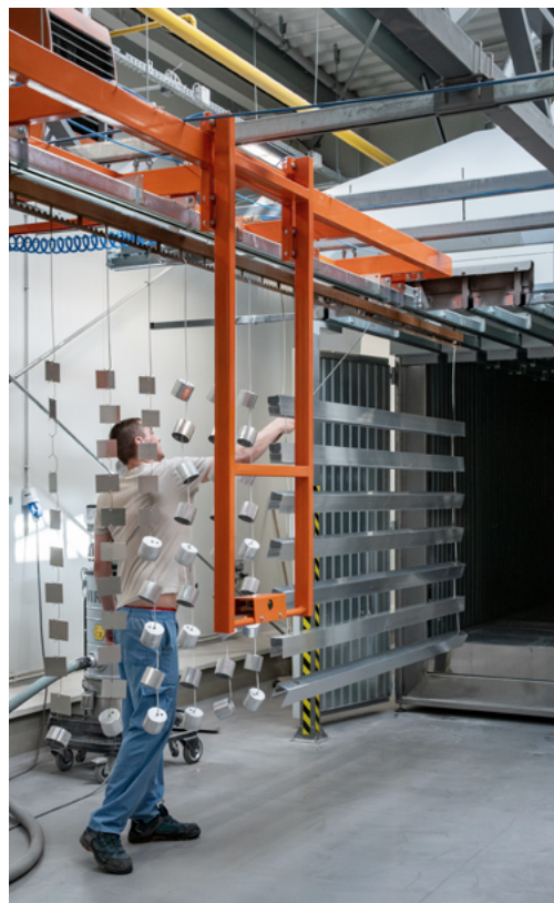
Photo 5. Illustration of the streamlined process for inserting a production batch into the oven, facilitated by the rail transport system.
