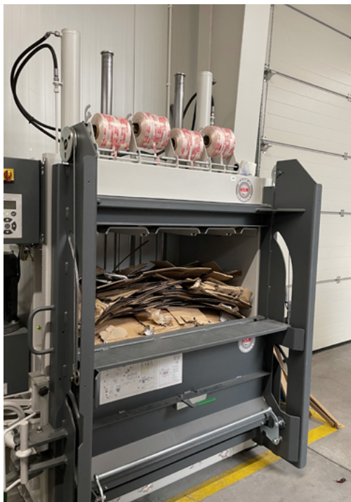
Photo 10. A machine designed for the crushing and packaging of paper waste at the production facility in Załuski.
