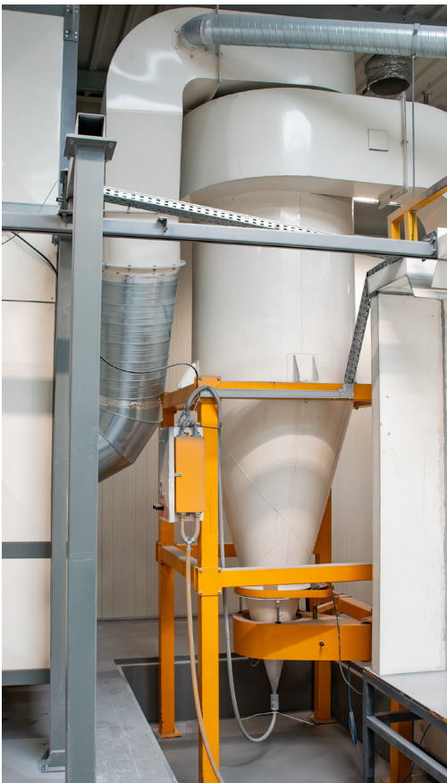
Photo 9. Advanced cyclone separator and fluid transport system integrated within the automated powder recovery loop at the Załuski complex.
