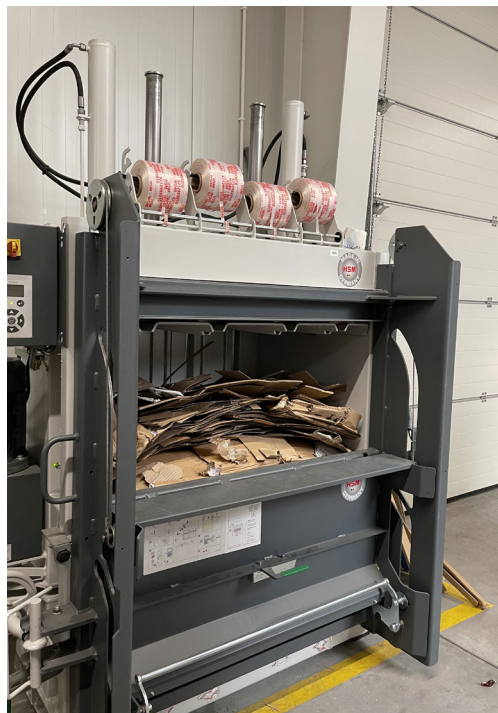
Photo 10. Heavy-duty vertical hydraulic cardboard baling and compaction system operational at the Załuski logistics hub.
