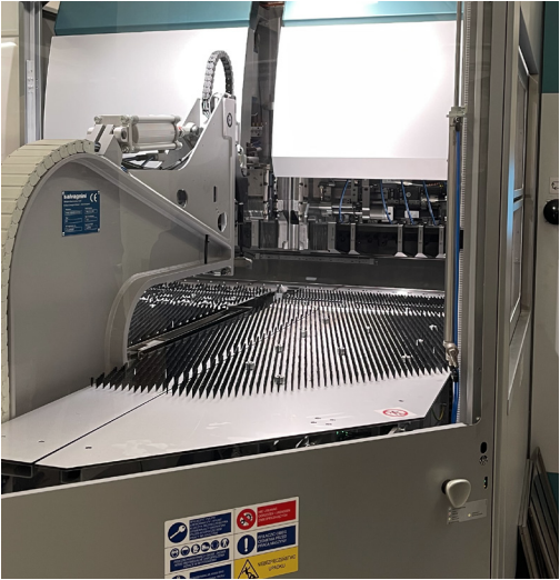
Photo 8. Automated CNC precision bending center, fully operational since 2024 and continuously driving throughput optimization at our Załuski manufacturing plant.
